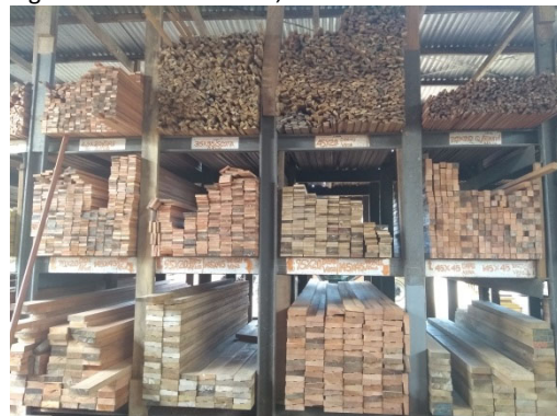
Figure 11: Dressed timber, in Honiara
